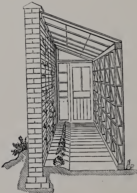
FIG. 35.—Interior perspective of Rivers' wall-tree cover. (Registered by Dennis & Co.)
